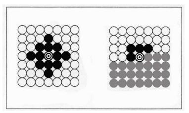
When (de)coding the original image using the reconstructed image as context, we can use two contexts, one for the reconstructed (left) and another one for the already (de)coded part (right). This allows better compression.
