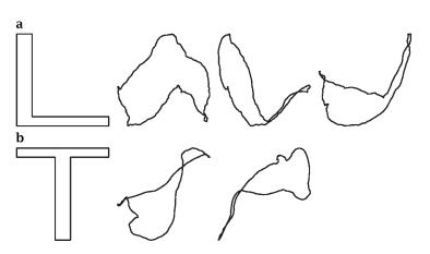
**Figure 19.9:** Importance of the phase for the description of shape with Fourier descriptors. Besides the original letters, three random modifications of the phase are shown with unchanged magnitude of the Fourier descriptors.
