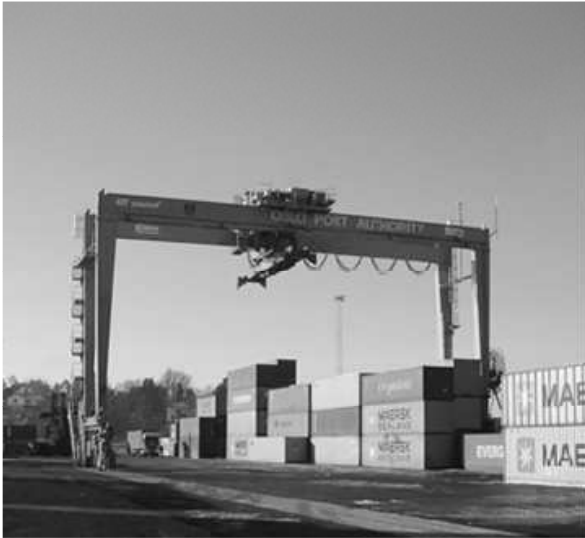
Figure 2. A Rubber-tired gantry crane (courtesy of Kalmar Industries).
