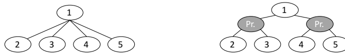
Fig. 9. Debugging tree (left) and its completely balanced version (right). The grey nodes are projection nodes.
